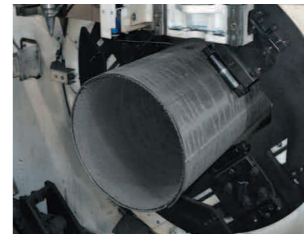
4-jaw roller chucking system supports workpiece material -even thin walled material can be handled with no problem
