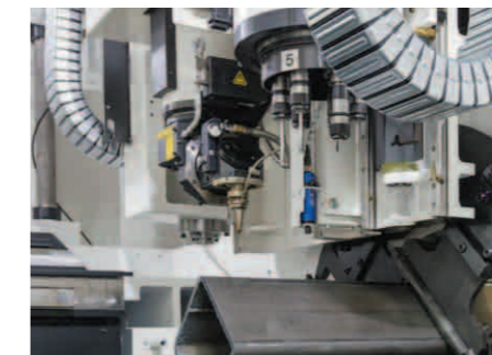
Tapping tools and touch sensor located next to cutting torch
