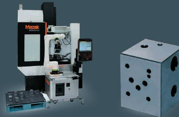
Vertical machining center with the Ez LOADER
