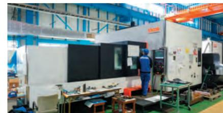
FJV-100/120 II that supports machining of large chambers
