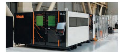
Newly installed OPTIPLEX 3015 FIBER 8.0 kW
