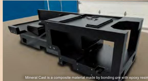
Mineral Cast is a composite material made by bonding ore with epoxy resin
