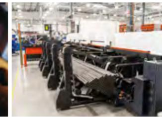
Large capacity bundle loader for pipe material
